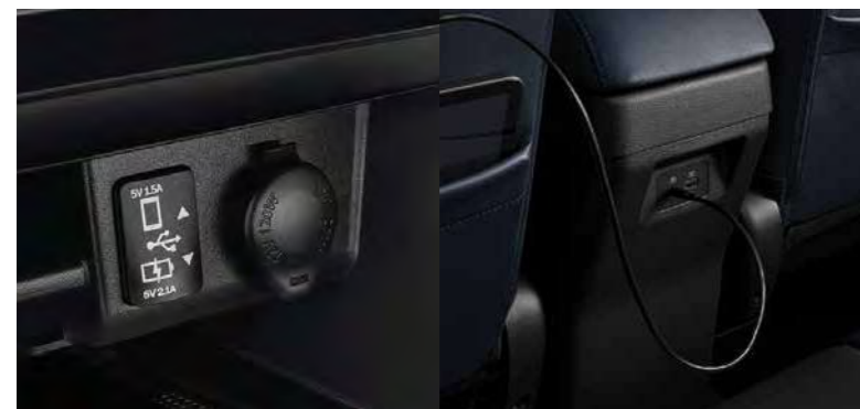
FRONT USB-A FOR DISPLAY AUDIO CONNECTIVITY AND 2 nd ROW SEAT USB-A AND USB-C CHARGER
