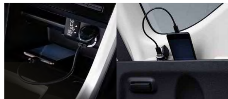
DC 12V ACCESSORY POWER SOCKET AT FRONT CONSOLE AND 3 rd ROW SEAT
